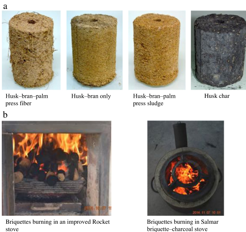
Fig. 2. (a) Different types of briquettes produced from husk-bran mixtures from Engelberg type mills and rice husk char; (b) burning of rice-husk briquettes in rocket and Salmar briquette-charcoal stoves.
