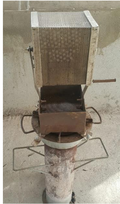
Figure 4. Pop rice (left) and prototype rice husk fueled pop rice marker (right)
