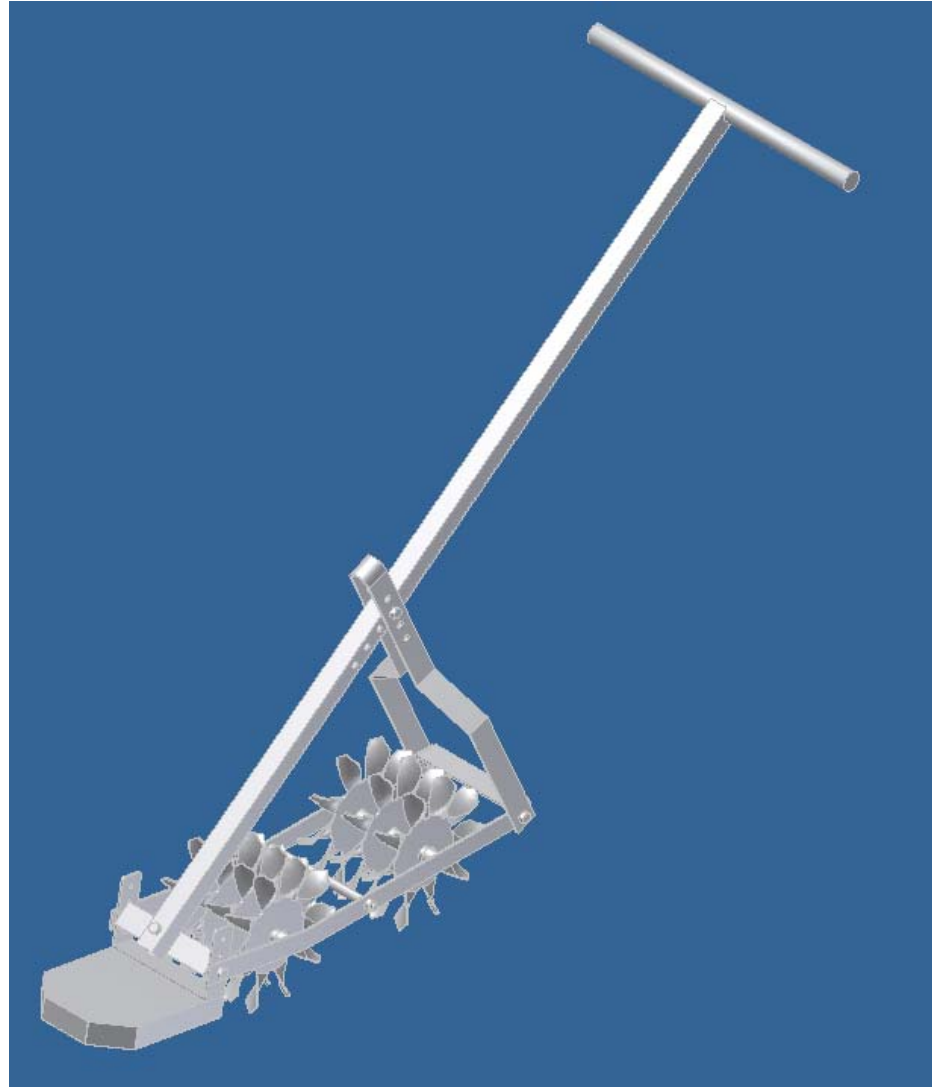
Figure 1A: Pictorial view of the Twisted-Spike Floating Weeder assembly
